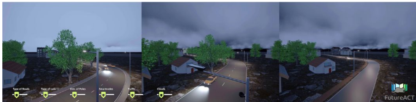
Figure 1: This is a demonstration for an application specific configurator. With the click of a mouse, you can change road classifications, pole and bracket dimensions or apply various lighting strategies in real time, like the Smartnodes light bubble
