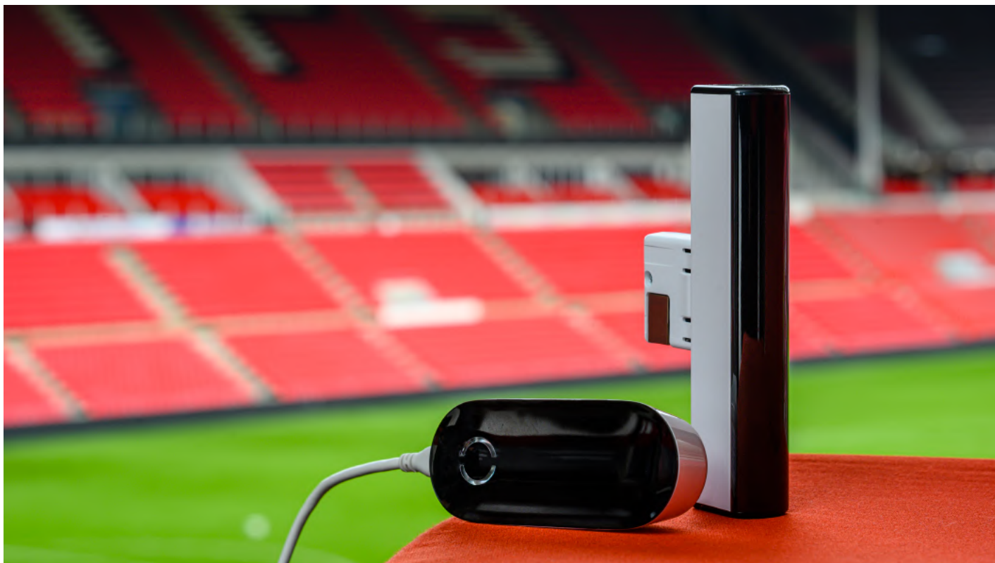
Figure 2: Access point and the LiFi endpoint, which are installed in the Philips stadium in Eindhoven
