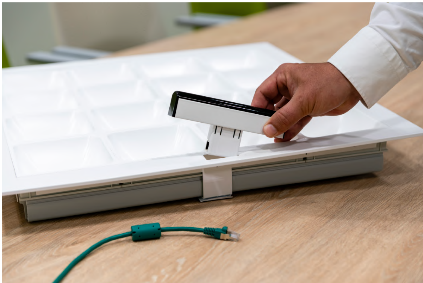
Figure 3: LiFi transceiver connects to an office luminaire
