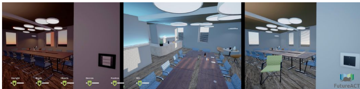
Figure 3: This project combines KNX controls, automatic blinds and a human centric lighting approach using the change of color, brightness and direction- all dependent on time, and offers results and configuration opportunities in real-time
