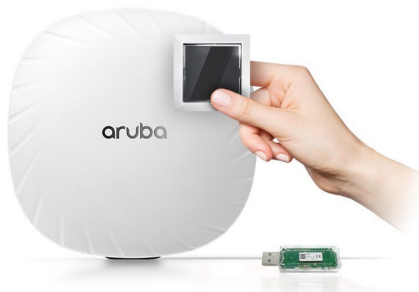
Figure 4: Using already existing Wi-Fi access points for IoT networks eliminates the need to install additional data network infrastructure.
