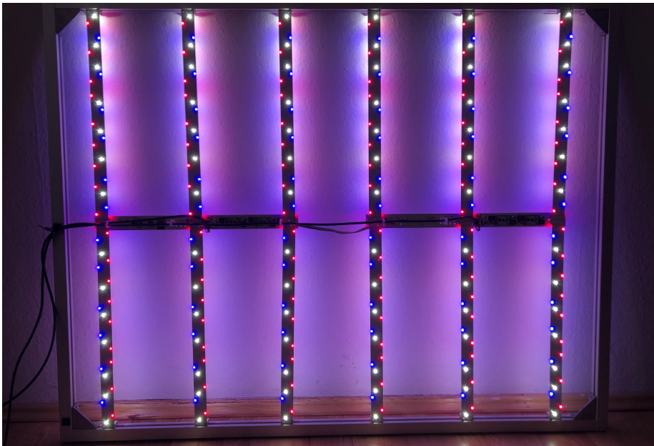
Figure 2: Light curtain with Würth Elektronik Horticulture Midpower LEDs of the WL-SMTW series and white LEDs of the SWTP series: a microcontroller enables flexible and dynamic light mixing. (Source: Agile Solutions)
