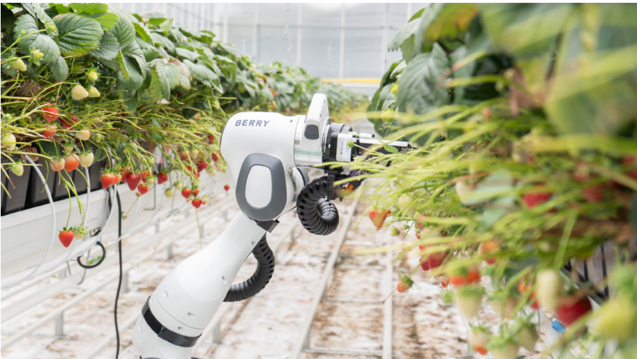
Figure 4: BERRY harvesting robot: With its LED lighting, the machine detects ripe fruit even under unfavorable lighting conditions. (Source: Organifarms)
