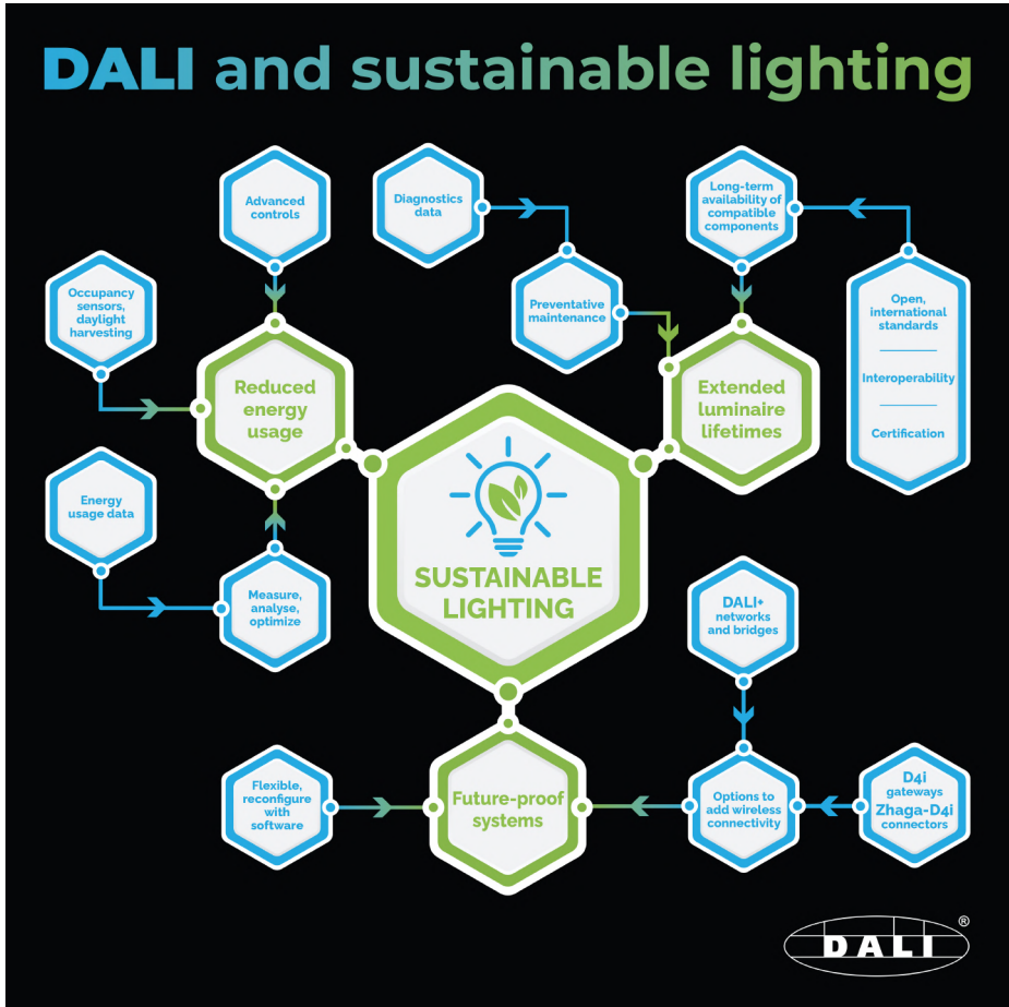
Figure 2: DALI can make important contributions to sustainable lighting systems via futureproofing, extended luminaire lifetimes and reduced energy usage.
