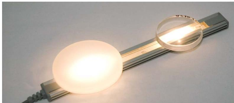
*Image 2 – Comparison of clear (UR5634) and diffusing (UR5635) polyurethane resins*
