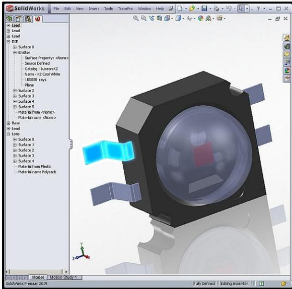
**Figure 11 – Luxeon LED as modeled as a surface source using the TracePro Bridge for SolidWorks**
