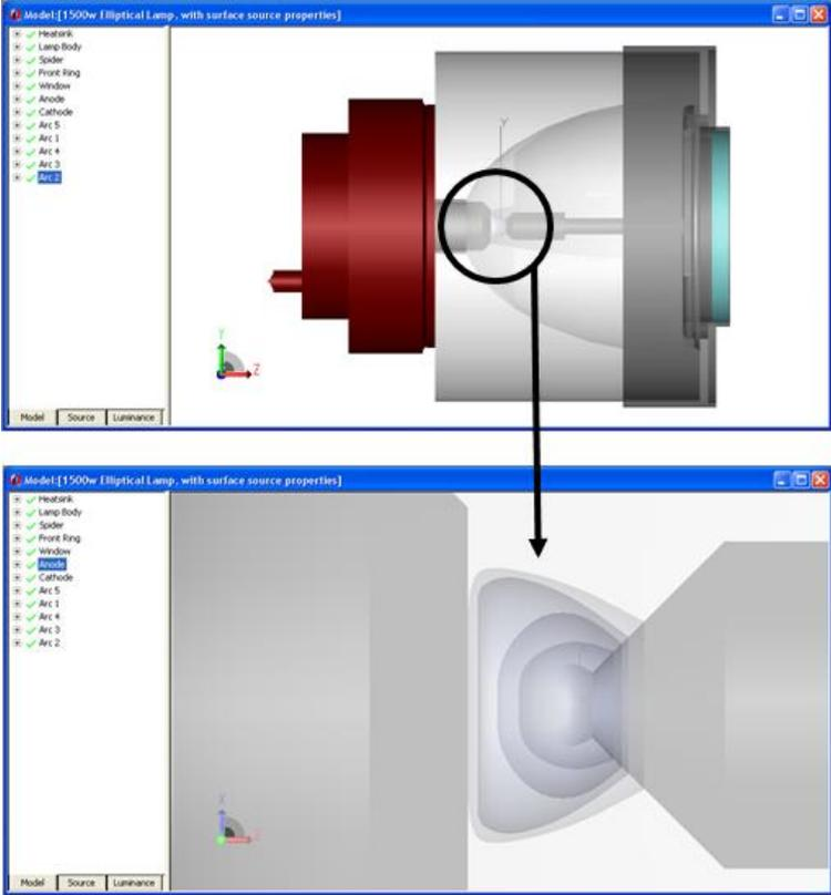
***Figure 10 - Arc model with surface source***
