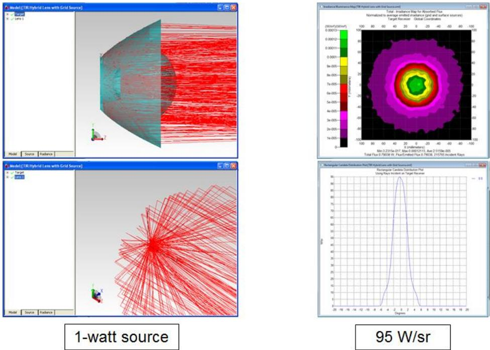
**Figure 5 - TIR hybrid lens with 1mm x 1mm grid source**
