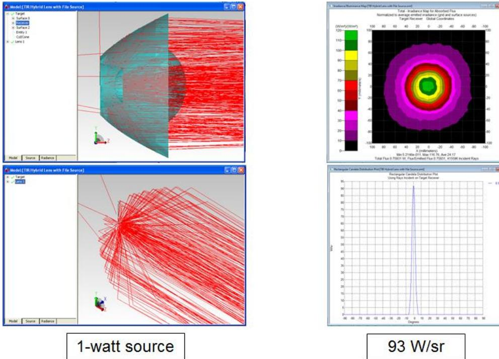
**Figure 7 - TIR hybrid lens with Ray File source**
